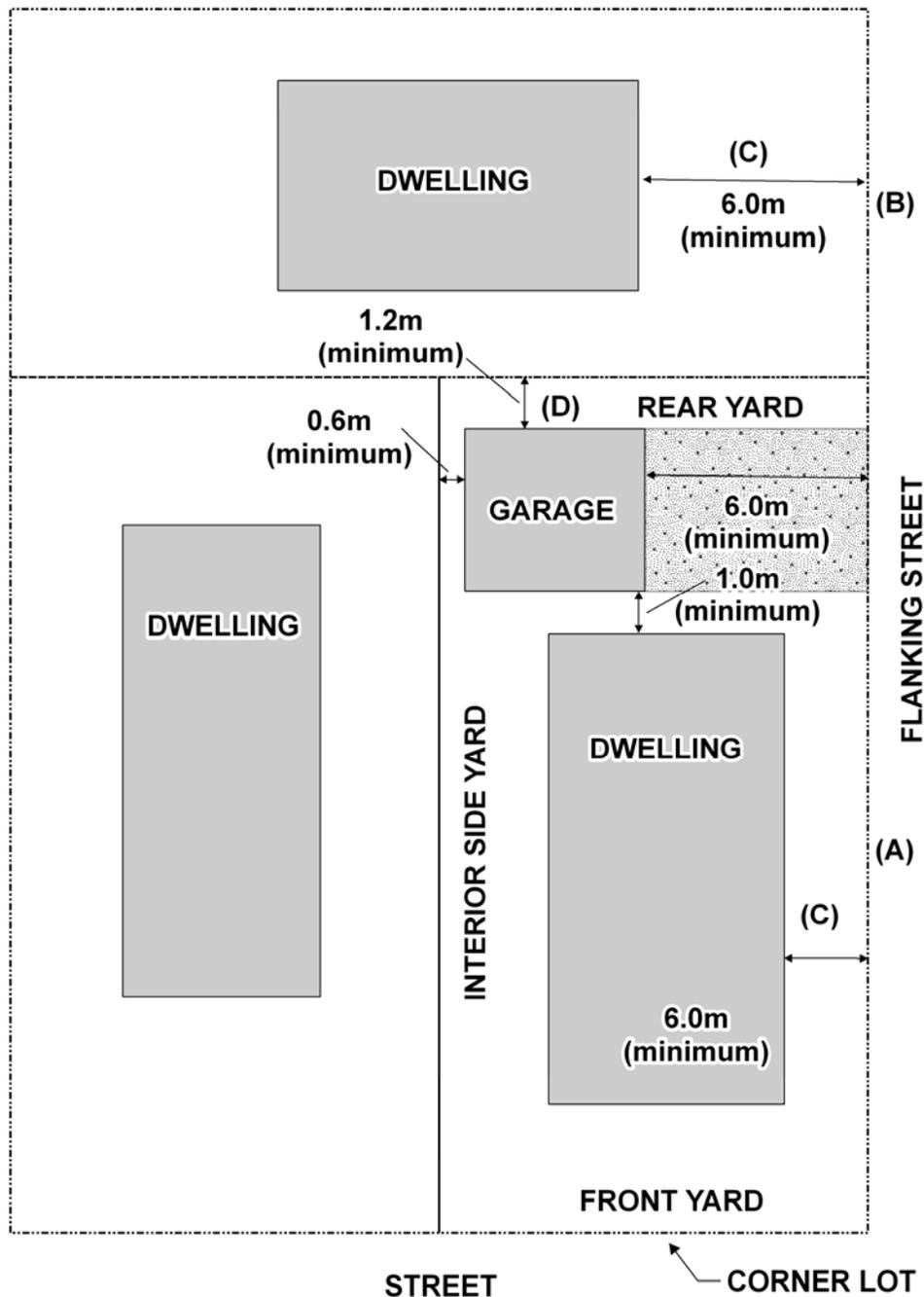
As shown in Figure 3, in any rear yard, a freestanding garage or other accessory building shall have a minimum building setback of 0.6m. No accessory building shall be closer than 3m to a flanking street. If a garage or carport has a vehicular entrance that faces the street, a minimum setback of 6m is required.
