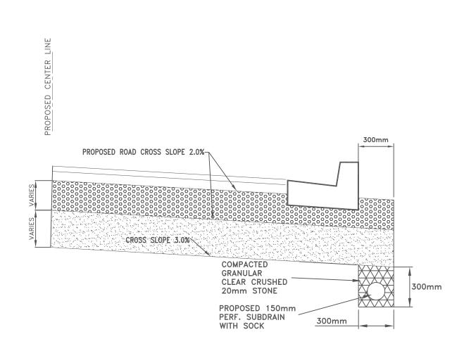
TYPICAL CROSS SECTION TO BE USED FOR DIAGRAMATIC VIEW ONLY
