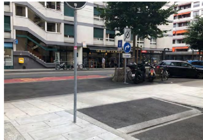
Figure 8: Continuous sidewalk in Geneva, Switzerland
