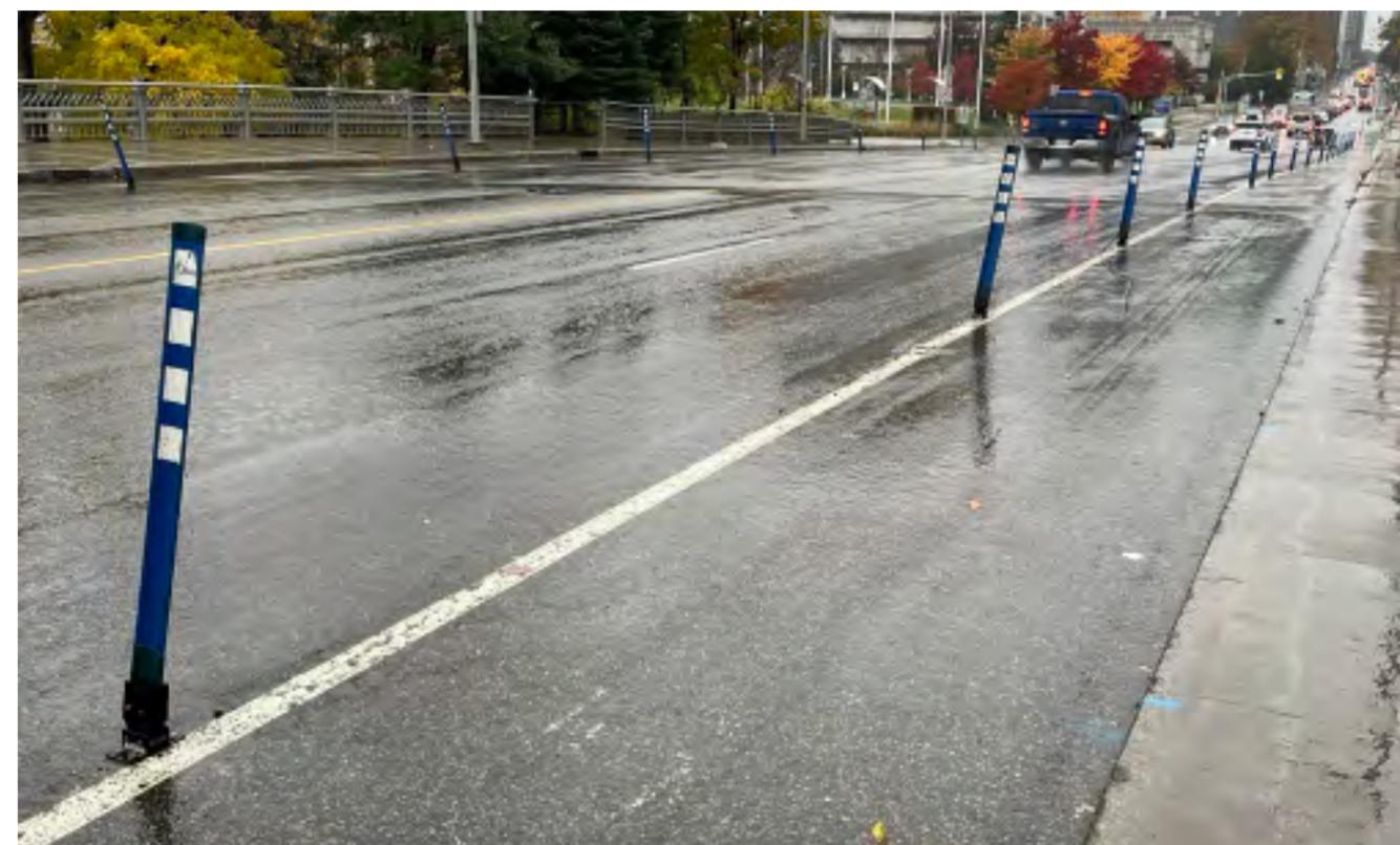
Figure 4: Flex posts on a unidirectional bike lane in Ottawa, CA
