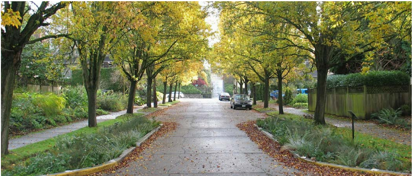
Curb extensions slow traffic, provide improved public safety, and slow stormwater run-off.
